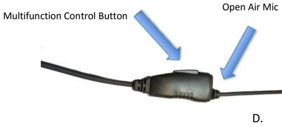
The Multifunction Control Button functions the same for the 1-wire and the 2-wire headset.
